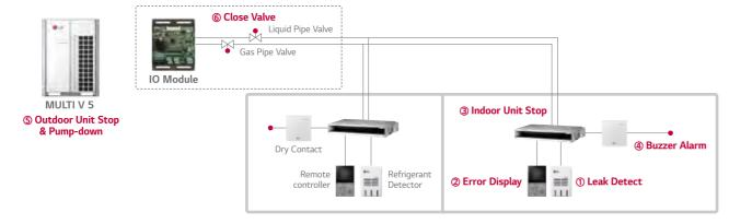
If the concentration of the refrigerant in the air exceeds 6,000 ppm more than 5 seconds, the function will be activated.
