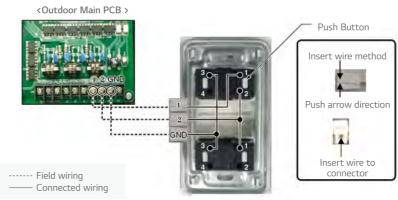
Connect Terminals (1, 2, GND) on the back side of the outdoor dry contact to terminals (1, 2, GND) of outdoor as shown below.
