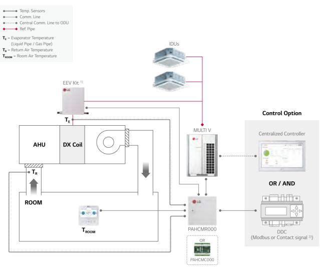
1) Multiple EEV kits can be applicable with multiple DX Coils and PAHCMR000s.
