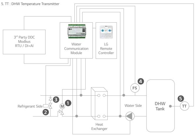
• 3rd party solenoid, non-return valve, heat exchanger, flow switch and DHW temperature transmitter (Optional) must be purchased separately. (Field supplied items)
