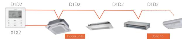
Note: when the ATOM Series indoor units connect to group controller WDC-120G/WK, the indoor units need to customize D1 D2 terminals. Group control is not available for Wall Mounted Series.
